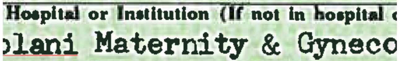
Figure 11. showing a mixture of grayscale and binary type on the same line.
